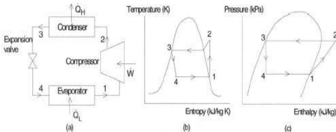
Figure 1 (a) A basic Vapor Compression refrigeration Cycle. (b) T-S diagram (c) its P-H diagram. [1]
