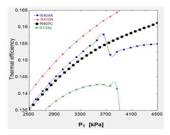
Figure 5: Variation thermal efficiency of organic rankine cycle with turbine inlet pressure
