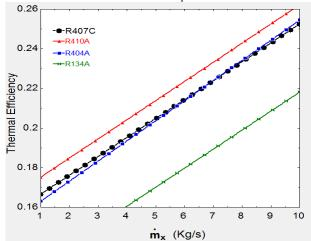
Figure 6: Variation of thermal efficiency with extraction mass from expander
