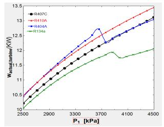
Figure 13: Variation work output of expander with the inlet pressure of expander
