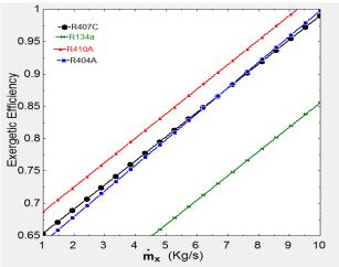
Figure 9: Variation of exergetic efficiency with mass extracted from expander
