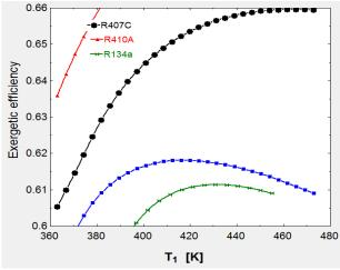
Figure 7: Variation of exergetic efficiency with inlet temperature of expander
