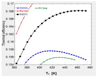
Figure 4: Variation of thermal efficiency of organic rankine cycle with expander inlet tempreture.
