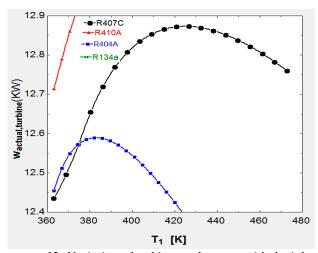
Figure 12: Variation of turbine work output with the inlet temperature of the expander
