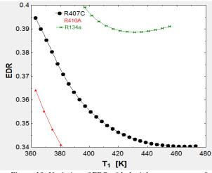
Figure 10: Variation of EDR with the inlet temperature of expander
