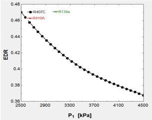
Figure 11: Variation of EDR with the inlet pressure of expander
