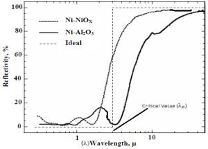
Figure 1: Shows the Wavelength  $(\lambda c)$  for Absorptivity (a) and Emissivity  $(\varepsilon)$ .
