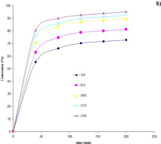
Figure 3: Evolution of the conversion level with time at different temperature- (a) Pd/C, (b) Ni
