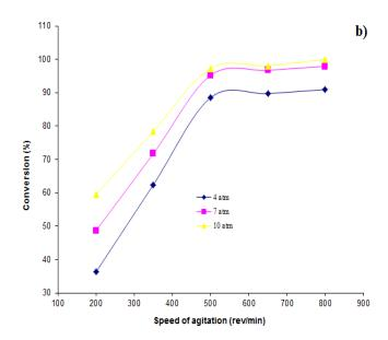
Figure 2: Evolution of the conversion level at different speed of agitation- (a) Pd/C, (b) Ni
