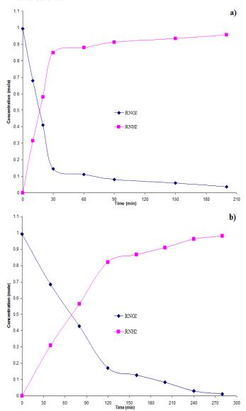
Figure 5: Dimethyl-nitrobenzene and dimethyl-aniline concentrations in solution verses time of reaction- (a) Pd/C (b) Ni
