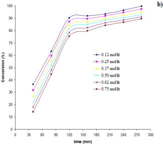
Figure 4: Evolution of the conversion level with time at different dimethyl-nitrobenzene concentration- a) Pd/C, (b) Ni
