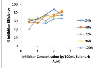
Figure 6: Effect of inhibitor concentration on inhibition efficiency.
