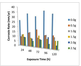
Figure 3: Effect of immersion period on corrosion rate
