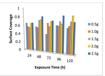
Figure 7: Effect of immersion period on surface coverage
