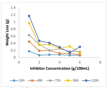
Figure 2: Effect of inhibitor concentration on weight loss
