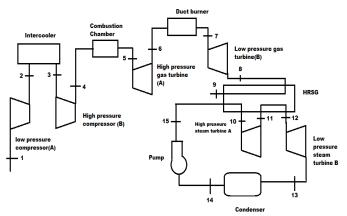
Figure 5: Combined cycle gas turbine (in present analysis)
