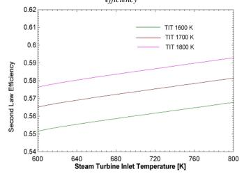
Figure 23: Effect of steam turbine inlet temperature on second law efficiency
