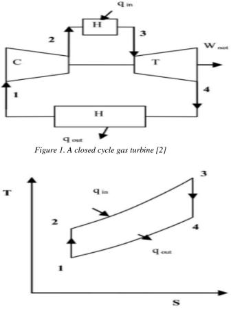
Figure 2: T-s diagram of Brayton cycle [2]
