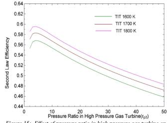
Figure 15: Effect of pressure ratio in high pressure gas turbine on second law efficiency
