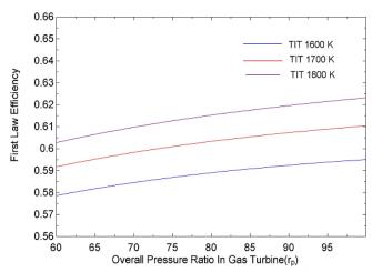
Figure 10: Variation of first law efficiency with overall pressure ratio in gas turbine
