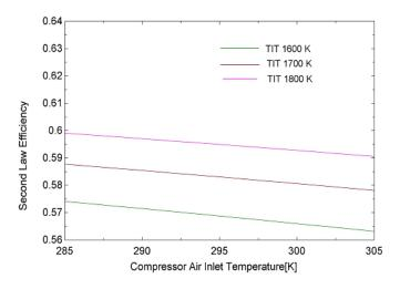
Figure 25: Effect of compressor inlet air temperature on second law efficiency
