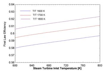
Figure 22: Effect of steam turbine inlet temperature on first law efficiency
