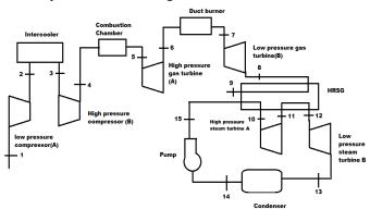
Figure 7: Modified combined cycle system
