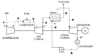
Figure 6: Simple Combined Cycle Gas Turbine System
