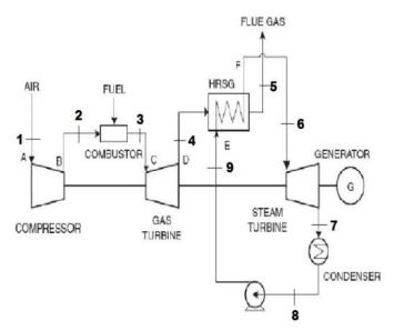
Figure 4: Simple combined cycle gas turbine
