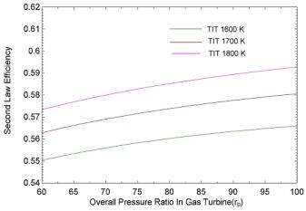
Figure 11: Variation of second law efficiency with overall pressure ratio in gas turbine
