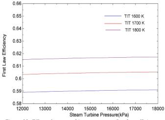
Figure 18: Effect of steam turbine pressure on first law efficiency
