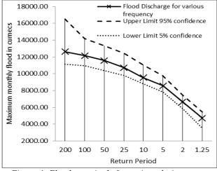
Figure 4: Flood magnitude for various design return period
