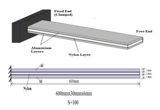
Figure 1: Aluminum-Nylon Laminated Composite Beam
