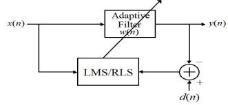
Figure 3. Block diagram for RLS adaptive equalizer
