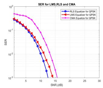
Figure 5: Results of RLS, LMS and CMA Equalization with QPSK
