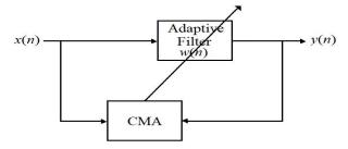
Figure 2: CMA Adaptive Algorithm Block Diagram
