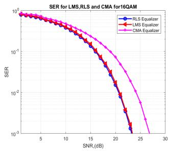
Figure 6: Results of RLS, LMS and CMA Equalization with 16-QAM
