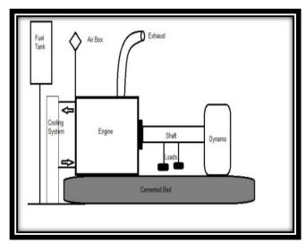
Figure 1: Schematic arrangement of experimental setup
