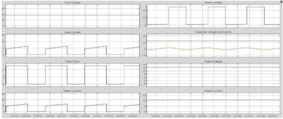
Figure 10: Waveform of the parameters of buck converter
