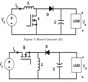
Figure 4: Buck-Boost Converter [6]
