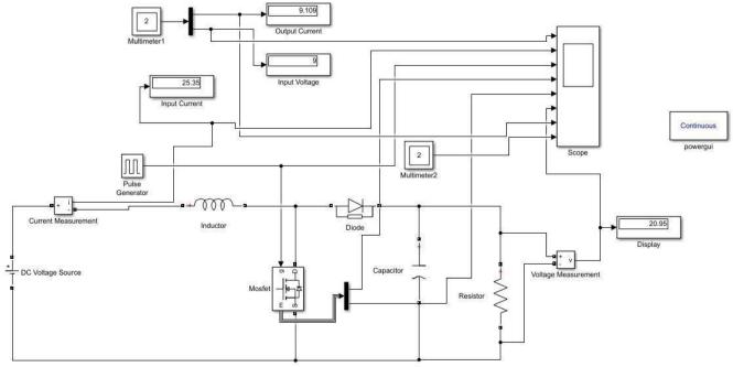
Figure 7: Simulation of Boost Circuit
