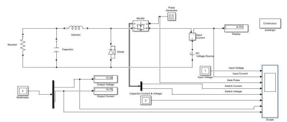
Figure 9: Simulation of Buck Circuit
