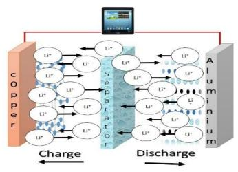
Figure 2: Electrochemical reaction of the Lithium-ion cell during charge and discharge process.
