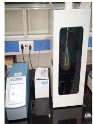
Figure 4: Probe type sonicator and Digital balance
