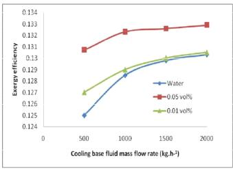
Figure 7: Variation of Exergy efficiency with cooling base fluid mass flow rate (kg.h<sup>-1</sup>)
