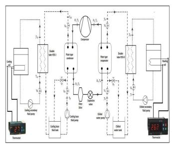
Figure 1: experimental test rig comprising of refrigerant
