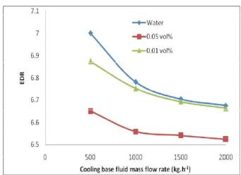
Figure 8: Variation of EDR with cooling base fluid mass flow rate  $(kg.h^{-1})$
