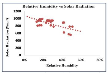
Figure 6: Variation of irradiance level with relative humidity
