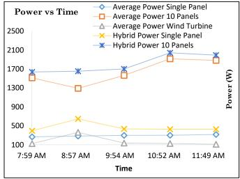
Figure 12: Power output measured with time for the three individual renewable energy systems compared with two hybrid systems.
