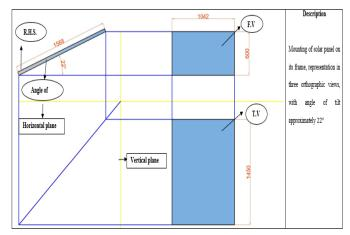
Figure 3: Orthogonal view of a single P.V panel in first angle of projection.
