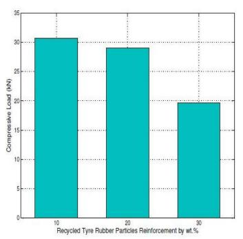
Figure 5: Compressive Load at break with variation of tyre rubber particles reinforcement by wt. percentage
