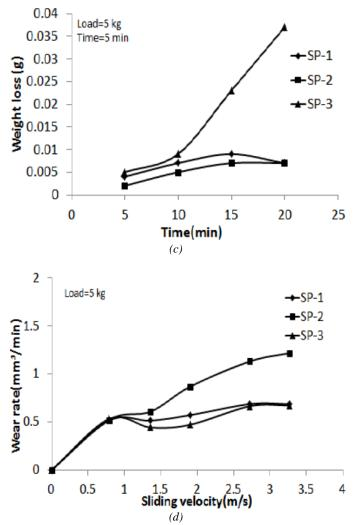
Figure 2: Different behavior of rubber dust composite, (a) Variation of coefficient of friction with load, (b) Variation of weight loss with speed, (c) Variation of weight loss with time, (d) Variation of wear rate with sliding velocity [7] Specimen-1- 10%, Specimen-2- 15% Specimen-3- 20% rubber dust by weight%
