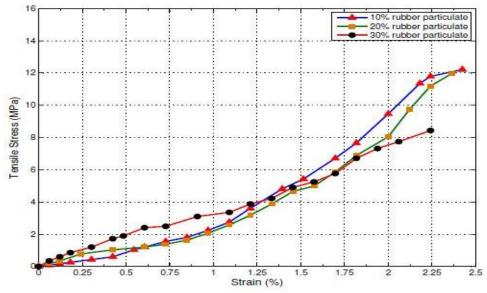
Figure 4: Stress/Strain curves for tensile test with variation of tyre rubber particles wt. percentage
