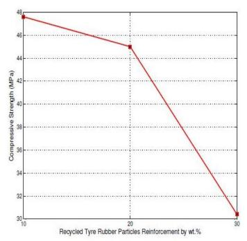
Figure 6: Compressive Strength with variation of tyre rubber particles reinforcement by wt. percentage
