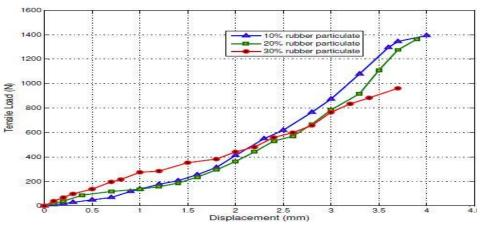
Figure 3: Load/Displacement curves for tensile test with variation of tyre rubber particles wt. percentage
