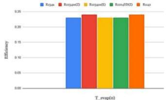
Figure 9: The graph compares the refrigerants based on their Efficiency at T\_evap(0). The results demonstrate that R1234ze(Z) and R1141 have higher Efficiency than R134a whereas R1234ze(E) and R1224YD(Z) have the same Efficiency than R134a.
