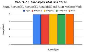
Figure 4: The graph compares the refrigerants based on their Comp Work at T\_cond(50). The results demonstrate that R1234ze(E), R1224YD(Z) and R1141 have higher Comp work than R134a whereas R1234ze(Z) have the same Comp work as R134a.
