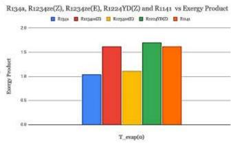
Figure 7: The graph compares the refrigerants based on their Exergy Product at T\_evap(0). The results demonstrate that R1234ze(Z), R1234ze(E), R1224YD(Z), and R1141 have higher Exergy Product than R134a.
