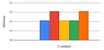
Figure 5: The graph compares the refrigerants based on their Efficiency at T\_cond(50). The results demonstrate that R1234ze(Z) and R1141 have higher Efficiency than R134a whereas R1234ze(E) and R1224YD(Z) have the same Efficiency than R134a.
