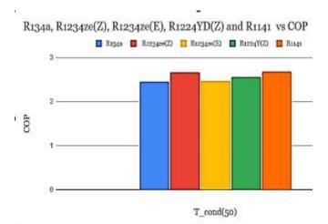
Figure 1: The graph compares the refrigerants based on their COP at T\_cond(50). The results demonstrate that R1234ze(Z), R1234ze(E), R1224YD(Z), and R1141 have higher COP than R134a.
