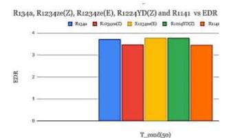
Figure 3: The graph compares the refrigerants based on their EDR at T\_cond(50). The results demonstrate that R1234ze(Z) and R1141 have lower EDR than R134a whereas R1234ze(E) and
