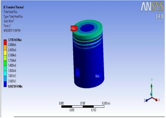
(b) Figure 5: Total heat flux for AlSiC10 (a) 3.0242e6 w/m<sup>2</sup> [11], (b) 3.15 w/m<sup>2</sup> (present value)
