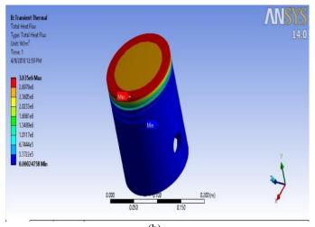
(b) Figure 4: Total heat flux for AlMgSi (a) 3.0325e6 w/m<sup>2</sup> [11], (b) 3.028 w/m<sup>2</sup> (present value)
