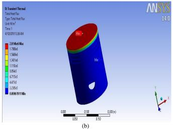
Figure 6: Total heat flux for (a) Structural Steel 3.0325e6 w/m<sup>2</sup>, (b) Cast Iron 3.028 w/m<sup>2</sup>
