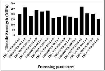
Figure 4: Variation of process parameters to the UTS.
