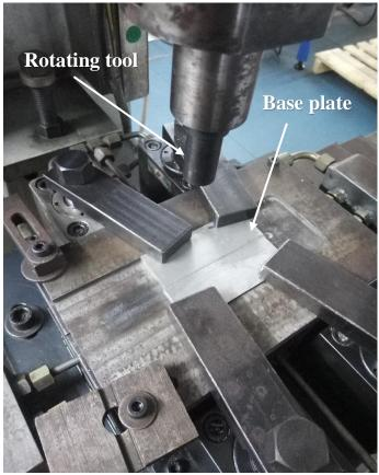
Figure 1: Friction Stir Welding
