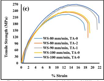
Figure 3: Stress strain diagram of welded joints of A6061 and AA7475, (a) 600 rpm, (b) 750 rpm, (c) 900 rpm
