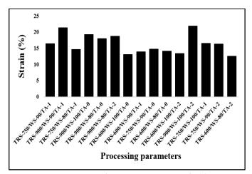
Figure 5: Variation of process parameters to the % strain
