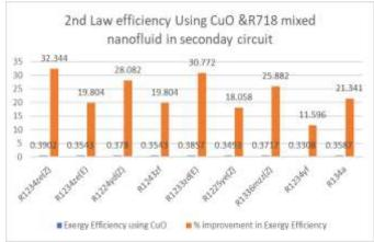
Figure 6: Second Law (exergy efficiency) performance of VCRS using eco-friendly refrigerant in the primary circuit and CuO+R718 mixed nanofluid in secondary circuit
