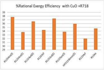
Figure 14: Rational Exergy efficiency(percentage) of VCRS using eco-friendly refrigerant in the primary circuit and CuO+R718 mixed nanofluid in the secondary circuit.
