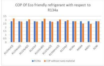
Figure 2: First law efficiency in terms of COP of VCR system using HCFO and HCFO refrigerants as compared with HFC-134a
