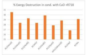
Figure 11: Exergy Destruction percentage in Condenser of VCRS using eco-friendly refrigerant in the primary circuit and CuO+R718 mixed nanofluid in secondary circuit.
