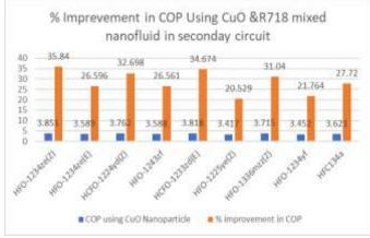
Figure 3: First law efficiency in terms of COP of VCR system using HFOs and HCFOs & HFCs refrigerants using CuO nano materials
