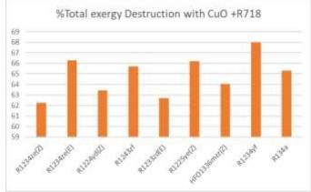
Figure 13: Total Exergy Destruction(percentage) of VCRS using eco-friendly refrigerant in the primary circuit and CuO+R718 mixed nanofluid in secondary circuit.
