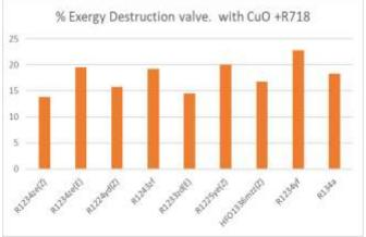
Figure 12: Exergy Destruction percentage in Valve of VCRS using eco-friendly refrigerant in the primary circuit and CuO+R718 mixed nanofluid in secondary circuit.
