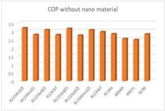
Figure 1: COP of VCRS using eco-friendly refrigerant in the primary circuit and R718 without nanoparticles in secondary circuit
