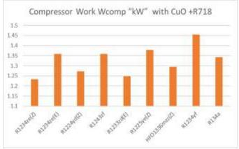
Figure 9: Compressor work of VCRS using eco-friendly refrigerant in the primary circuit and CuO+R718 mixed nanofluid in secondary circuit.
