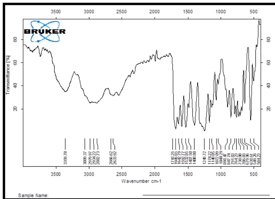
Figure 2: FTIR for derivative A.
