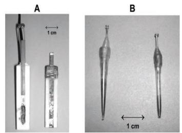
Figure 2: Some novel construction types of electrode holders for carbon paste. [91]
