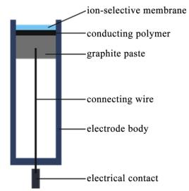
Figure 1: Assembly of the ion-selective electrode based on graphite paste [90]
