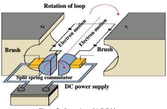
Figure 2: Operation of A DC Motor
