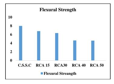
Figure 2-Variation of flexural strength with % replacement of RCA
