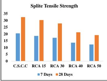
Figure 3- Variation of split tensile strength with % replacement of RFA
