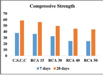
Figure 1- Variation of compressive strength with % replacement of RCA
