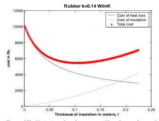
Figure 12b: Variation of total cost, cost of heat loss and cost of insulation with thickness of insulation for rubber material
