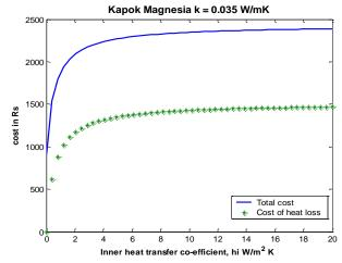
Figure 2b: Variation of total cost, cost of heat loss with inner heat transfer coefficient for kapok magnesia material
