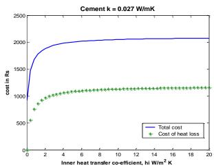
Figure 3a: Variation of total cost, cost of heat loss and cost of insulation with inner heat transfer coefficient for cement material
