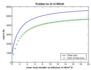
Figure 12a: Variation of total cost, cost of heat loss with inner heat transfer coefficient for rubber material
