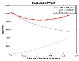
Figure 14b: Variation of total cost, cost of heat loss and cost of insulation with thickness of insulation for plastic material
