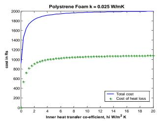
Figure 8a: Variation of total cost, cost of heat loss with inner heat transfer coefficient for polystrene material
