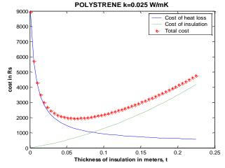
Figure 8b: Variation of total cost, cost of heat loss and cost of insulation with thickness of insulation for polystrene material
