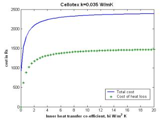
Figure 10a: Variation of total cost, cost of heat loss with inner heat transfer coefficient for cellotex material
