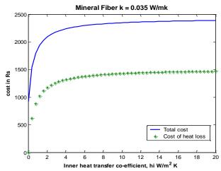
Figure 15a: Variation of total cost, cost of heat loss with inner heat transfer coefficient for mineral fibre material
