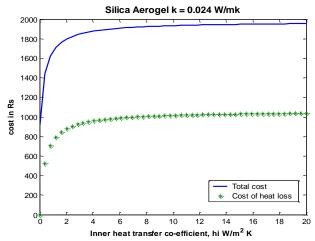
Figure 6 a: Variation of total cost, cost of heat loss with inner heat transfer coefficient for silica aerogel material
