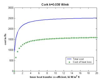
Figure 1(a): Variation of total cost, cost of heat loss with inner heat transfer coefficient for cork material
