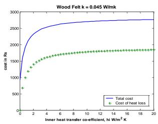
Figure 9(a): Variation of total cost, cost of heat loss with inner heat transfer coefficient for wood felt material
