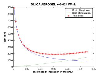
Figure -6b: Variation of total cost, cost of heat loss and cost of insulation with thickness of insulation with thickness of insulation for silica aerogel material
