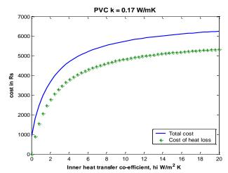
Figure 7a: Variation of total cost, cost of heat loss with inner heat transfer coefficient for PVC material
