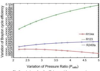
Fig 8 variation of cycle efficiency with pressure ratio
