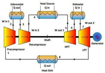
Figure 4: Layout of Brayton cycle with Intercooler and Re-heater
