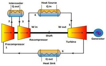
Figure 2: Brayton cycle with intercooling
