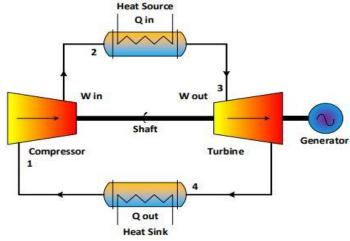
Figure 1: Schematic Diagram of Simple Brayton cycle
