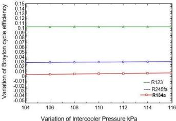
Figure 5: variation of cycle efficiency with intercooler pressure
