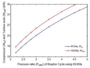
Fig 12 variation of compressor and turbine works with pressure ratio using R245fa
