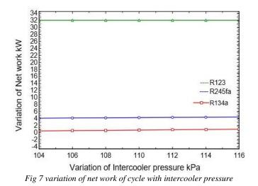
Fig 7 shows the outcome of net work by varying the intercooler pressure. As per the figure by increasing the intercooler pressure the net work is also increasing for R245fa and R134a but it is constant for R123. From fig.7 the Brayton cycle net work at intercooler pressure 106kPa is 32.04 kW, 4.217 kW and 0.6055 kW for fluid R123, R245fa and R134a respectively.
