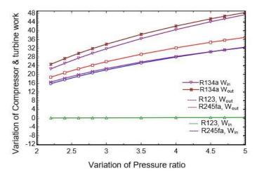
Fig 9 variation of compressor and turbine works with pressure ratio
