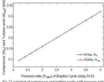
Fig 13 variation of compressor and turbine works with pressure ratio using R123
