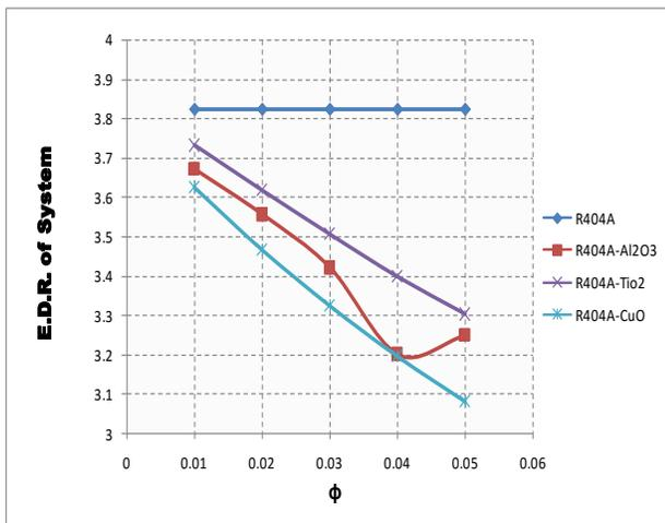
Figure: 3 Variation of Exergy destruction ratio with volume fraction ( $\phi$ ) of VCRS with R404A using different nano particles [24]
