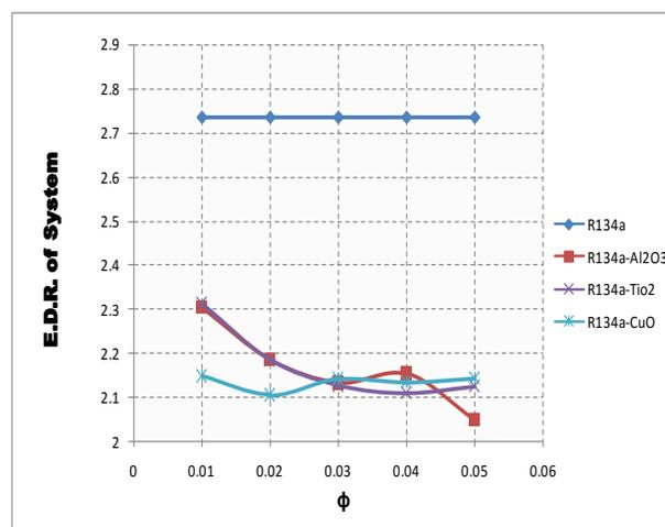
Figure: 1 Variation of Exergy destruction ratio with volume fraction ( $\phi$ ) of Vapour Compression Refrigeration System with R134a using different nano particles [24]
