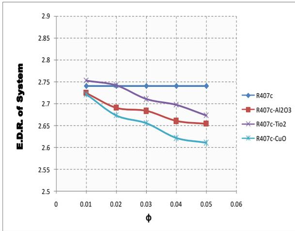
Figure: 2 Variation of Exergy Destruction ratio with volume fraction ( $\phi$ ) of Vapour Compression Refrigeration System with R407c using different nano particles [24]
