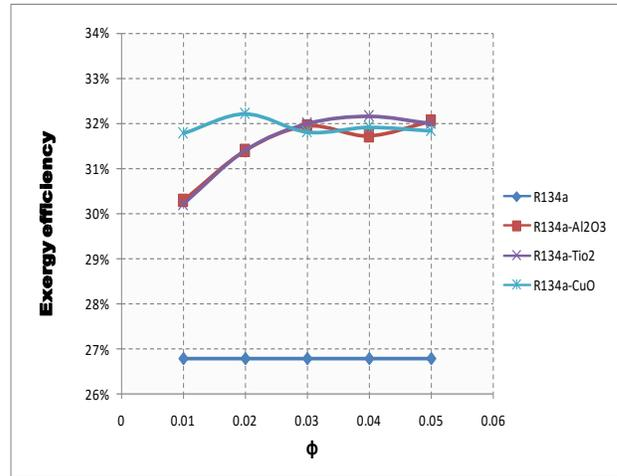
Figure: 4 Variation of Exergy Efficiency with volume fraction ( $\phi$ ) of Vapour Compression Refrigeration System with R134a using different nano particles [25]
