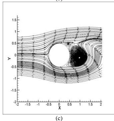
Figure 3:- Streams lines at  $Re = 200$  for (a)  $\alpha = 0^\circ$ , (b)  $\alpha = 5^\circ$ , (c)  $\alpha = 10^\circ$
