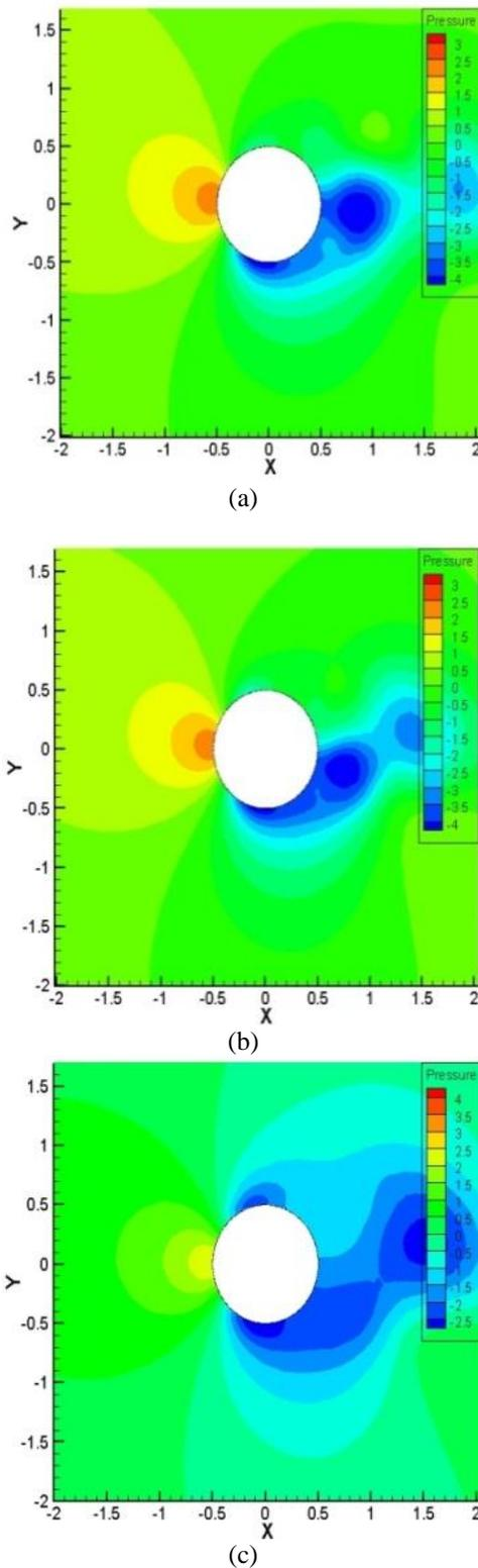
Figure 8:- Pressure contours at  $Re = 1000$  for (a)  $\alpha = 0^\circ$ , (b)  $\alpha = 5^\circ$ , (c)  $\alpha = 10^\circ$
