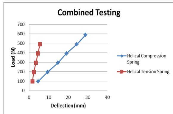
Figure 3:- Variation between load and Deflection for helical compression spring
