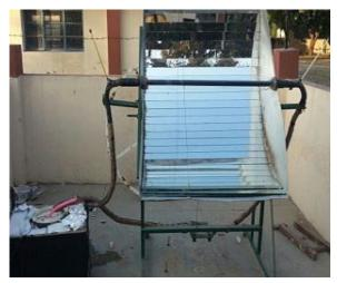
Figure: 2: Experimental set up of parabolic through collector at Thapar University, Patiala
