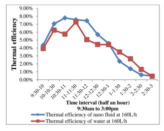
Figure. 7 variations in thermal efficiency with respect to time
