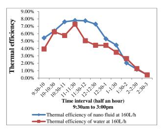
Figure. 9 variations in thermal efficiency with respect to time
