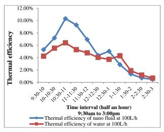
Figure. 10 variations in thermal efficiency with respect to time
