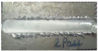
Figure 2(c): Double pass on the third Al workpiece with SiC
