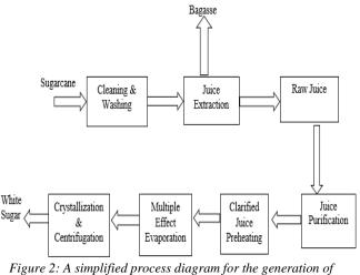
ure 2: A simplified process diagram for the generation sugarcane bagasse [17].
