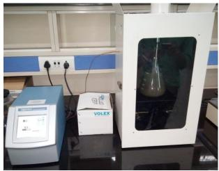
Figure: 6 Probe type ultrasonicator
