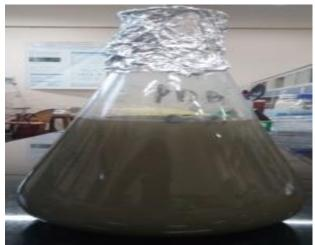
Figure: 12 Nano particle settlement after12 hours
