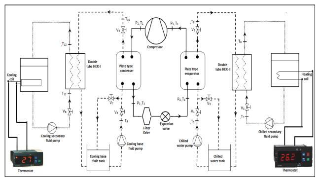
Figure: 1 Experiment test rig of vapour compression refrigeration system
