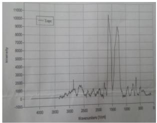
Figure: 4 Raman analysis of silver nanoparticles
