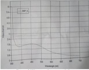
Figure: 3 UV spectrophotometer of silver
