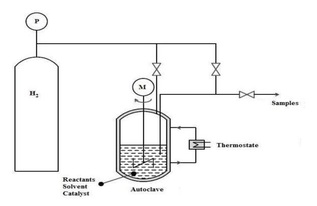
Figure 1: Experimental set-up for the liquid hydrogenation of dimethyl-nitrobenzene
