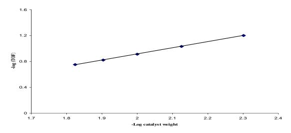
Figure 9: log (TOF) vs. log catalyst weight (363 ° K , H<sub>2</sub> pressure 1000 kPa)
