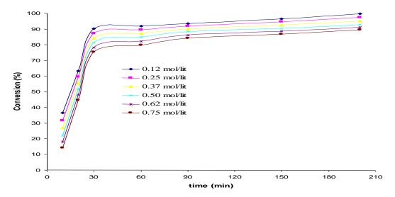
Figure 2: Evolution of the conversion level with time at different dimethyl-nitrobenzene concentration
