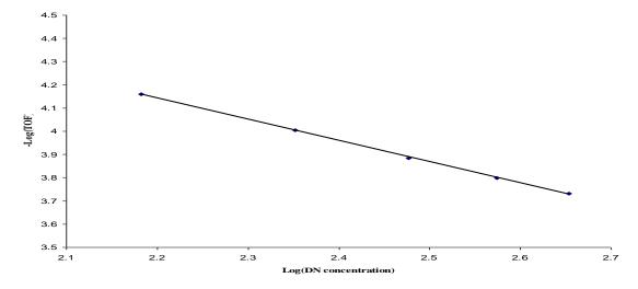
Figure 7: log (TOF) vs. log dimethyl-nitrobenzene concentration (H<sub>2</sub> pressure 700 kPa, catalyst loading 10 kgm<sup>-3</sup>, 363
