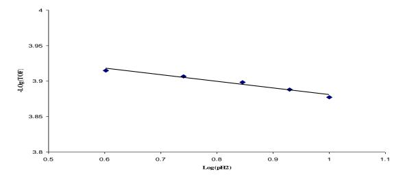
Figure 8: log (TOF) vs. Log hydrogen pressure (initial DN concentration 0.5 kmolm $^{-3}$ , Catalyst loading 10 kgm $^{-3}$ , 363  $^{\circ}K$ )
