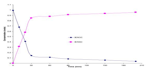
Figure 3: Dimethyl-nitrobenzene and dimethyl-aniline concentrations in solution verses time of reaction <sup>0</sup>K)
