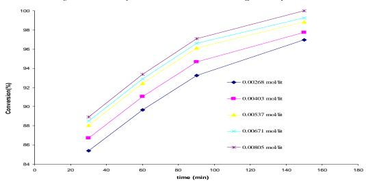
Figure 6: Evolution of the conversion level with time at different weight of catalyst
