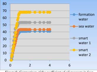
Figure 6: Comparison of the coefficient of oil recovery in four stages in terms of the volume of injectable solutions
