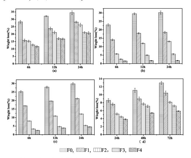
(a) Anhydrous ethanol, (b) Cyclohexane, (c) Petroleum ether, (d) Activated carbon Figure 2: Weight losses of PVC films after migration and exudation testing [12]
