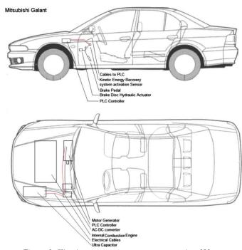
Figure 1: Kinetic energy recovery system overview [8]
