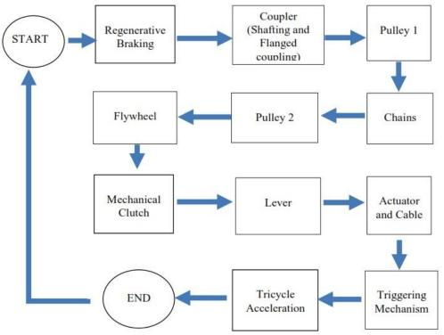
Figure 1: Flowchart diagram of the flywheel kinetic energy recovery system [9]
