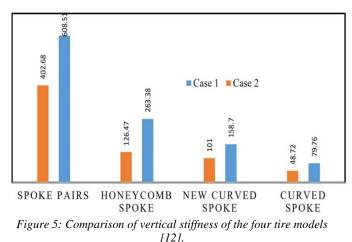
The Static Load Deflection process measures the displacement of the hub center when a load is applied to evaluate tyre stiffness, where vertical stiffness is defined by Eq (1). Where F is the vertical force (3000 N);  $\delta$  is the vertical deflection of the hub center.
