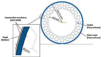
Figure 1: Different parts and dimensions of NPT [12].
