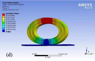
Figure 4: Deflection of air less tyre, (a) Honey Comb Structure, (b) Spoke type Structure, (c) Triangular type Structure, (d) h diamond Structure [15]
