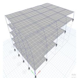
Figure 2: Mode shape 1 of Model 2 with natural period of 0.179
