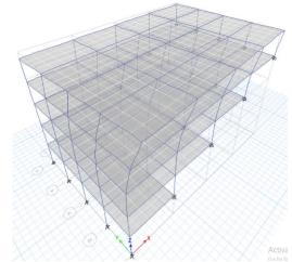
Figure 1: Mode shape 1 of Model 1 with natural period of 0.29
