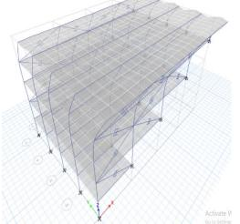
Figure 3: Mode shape 1 of Model 3 with natural period of 0.255
