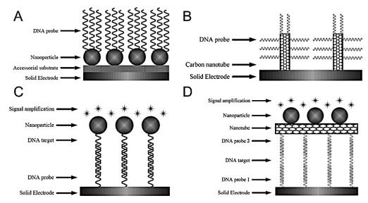
Figure 2: Principles for nanometrial sensor in DNA probs (a). electrode coated(b). probe labeling(c). target labeling (d). signal reported [31]
