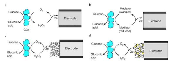
Figure 1: General GOx electrochemical biosensors (a,b). GOx layer (c,d). nanocomposites working together[22]
