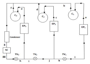
Fig.2 (a) Schematic diagram of multiple evaporators at different temperatures with individual compressors and multiple expansion valves
