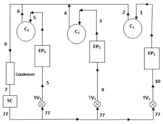
Figure 1 (a) Schematic diagram of multiple evaporators at different temperatures with individual compressors and individual expansion valves
