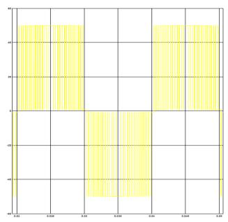
Figure 10: Level Output Waveform (PWM)
