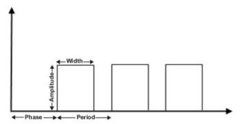
Figure 4: Explanation of wave measurements
