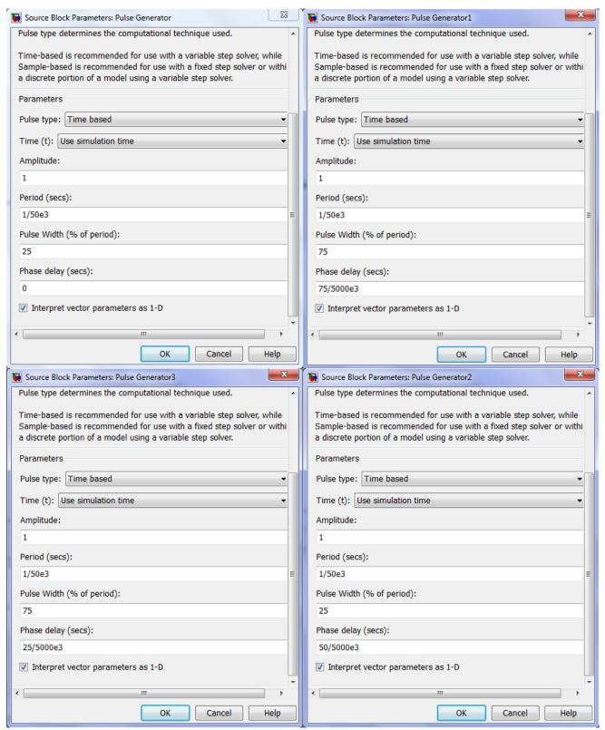
Figure 6: Switches Source Block Parameters
