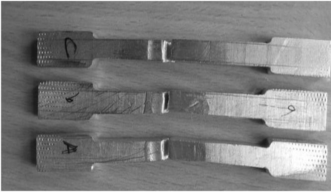
Figure 10: After tensile testing of welded material specimens
