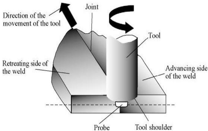
Figure 1: Two discrete metal workpiece butted together, along with the tool (with a probe)
