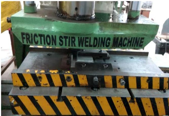
Figure 3: Friction Stir Welding set up
