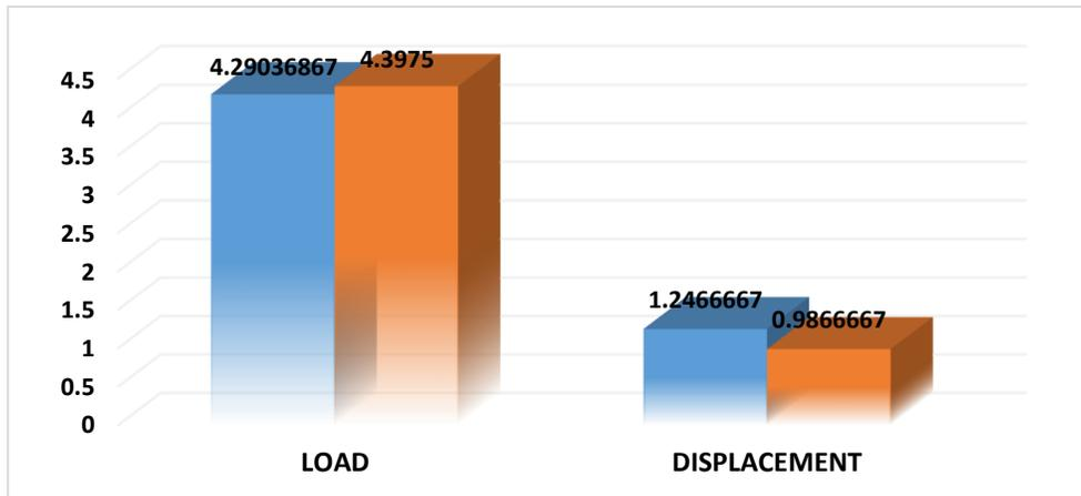
Figure 11: Variation in load and displacement of both before and after welding of FSW on specimen Al-2029
