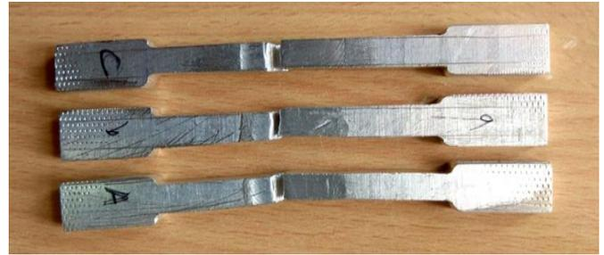
Figure 8: Tensile testing of specimen by UTM machine up to fracture point
