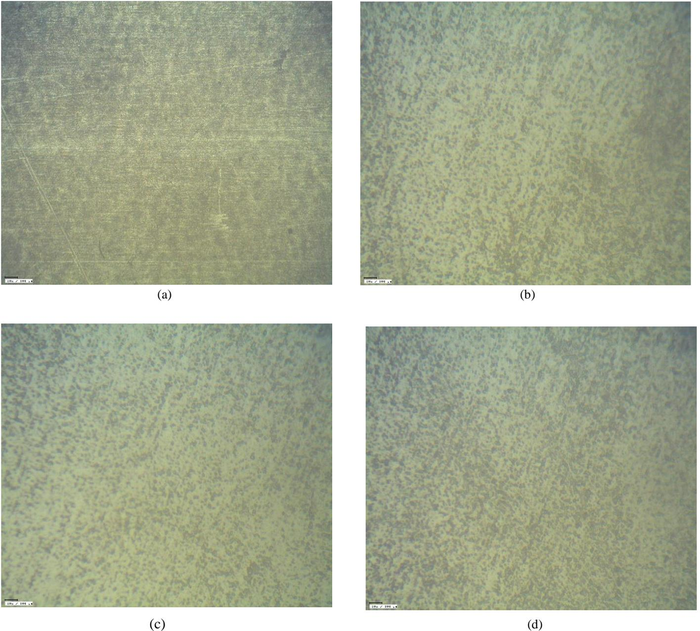
Figure 15: Optical Microstructure of FSW of Al-2029, (a) Stir zone, (b) HAZ, (c) Base zone (d) Weld nugget
