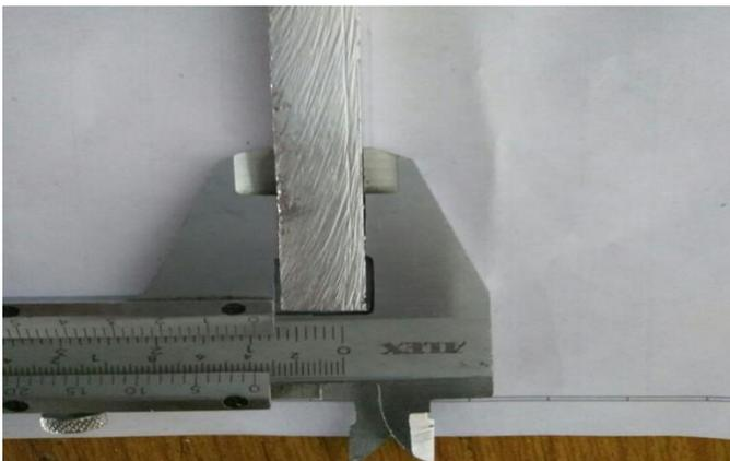
Figure 7: Dimension inspection by Vernier calliper
