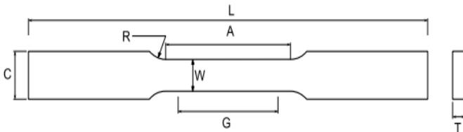
Figure 5: Tensile test specimen
