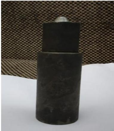
Figure 2: Tool of mild steel for FSW
