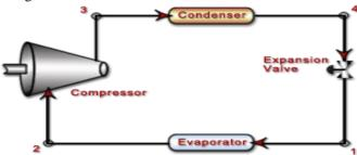
Figure 1: Vapour compression refrigeration system [1]
