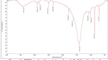
Figure 8: FTIR peaks of precipitated peak CaCO3 of isolate 9
