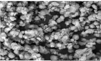
TM3030 1334 2018/03/12 11:17 HL D5.7 ×4.0k 20 μm Plate 5: SEM image of crystal precipitated by isolate I
