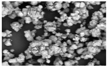
$\overline{TM}$ 3030 1330 2018/03/12 11:06 HL D5.6 x4.0k 20 µn Plate 7: SEM image of crystal precipitated CaCO<sub>3</sub> by isolate 6
