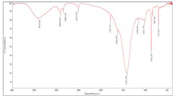
Figure 5: FTIR peaks of precipitated CaCO<sub>3</sub> of isolate 1
