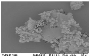
Plate 8: SEM image of precipitated CaCO<sub>3</sub> crystal of isolate 9
