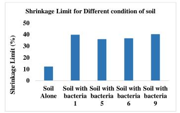
Figure 10: Different range of values for Shrinkage Limit
