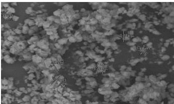
TM3030 1355 2018/03/12 12:29 HL D5.6 ×3.0k 30 μm Plate 4: SEM image of Control crystal of precipitated CaCO3
