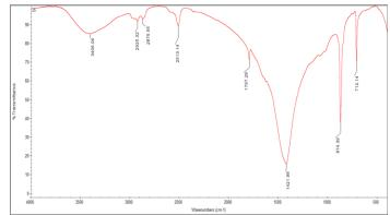
Figure 6: FTIR peaks of precipitated peak CaCO<sub>3</sub> isolate 5
