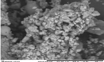
TM3030 1343 2018/03/12 11:46 HL D5.6 ×3.0k 30 μm Plate 6: SEM image of crystal precipitated CaCO3 by isolate 5
